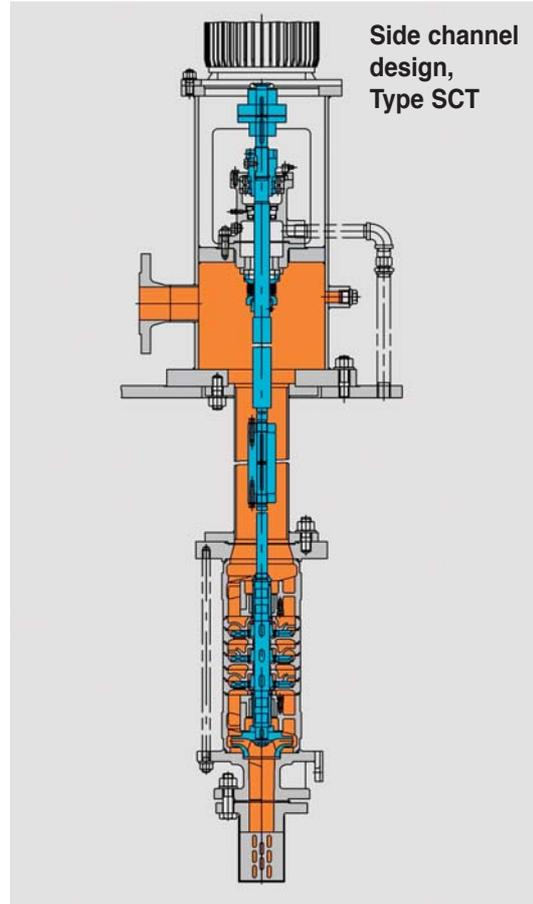
Special design for low flow and high head applications. Pump body and performance table is identical to Type SC (see corresponding leaflet).
