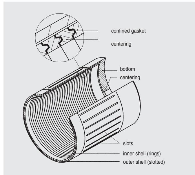
This "low-loss" containment shell is recommended especially for driving power
