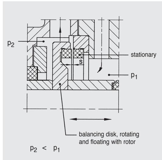
connected with the pressure side of the first pump stage via an external auxiliary pipe. According to the rotor position and the adjusting gap  $S$ , a counter force is created by the differential pressure between front and rear side of the balancing disk. This counter force acts against the residual load towards the containment shell such that no thrust loads occur. No thrust bearings are required. The start-up rings keep the pump shaft in position during start-up and shut-off.
